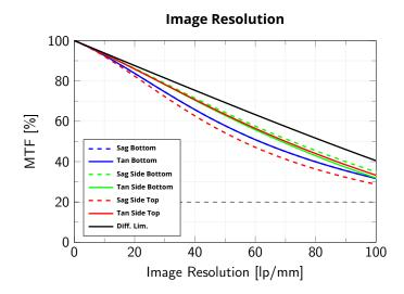
Modulation Transfer Function (MTF) vs. Image Resolution (wavelength range 486 nm - 656 nm), wf/N=8, of cylindrical object of diameter 30 mm and height of 20 mm
